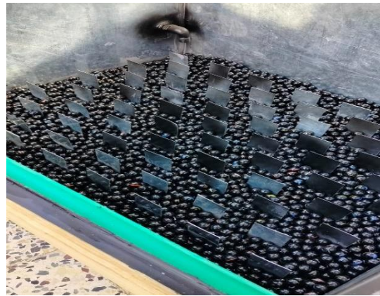
Figure 4: The porous media (black glass balls) in the basin of the MSS-FPPCM system
