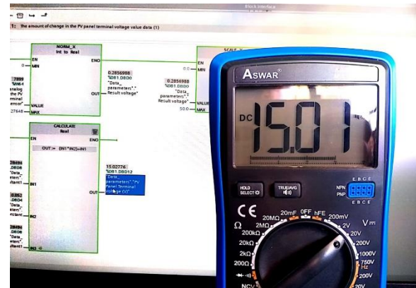
Figure 2 (a). The correlation between the PLC readings and the voltage sensor's measurements taken with a voltmeter
