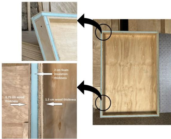
Figure 6. The frame of the solar collector.
