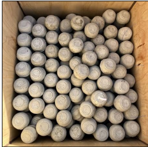
Figure 7. Cement mortar molds, a photo from the top of the storage unit.
