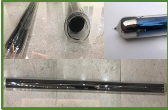
Figure 4: Evacuated glass absorber tube.
