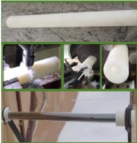
Figure 5: Stages of manufacturing a thermal Teflon grip for the ends of the absorber tube.
