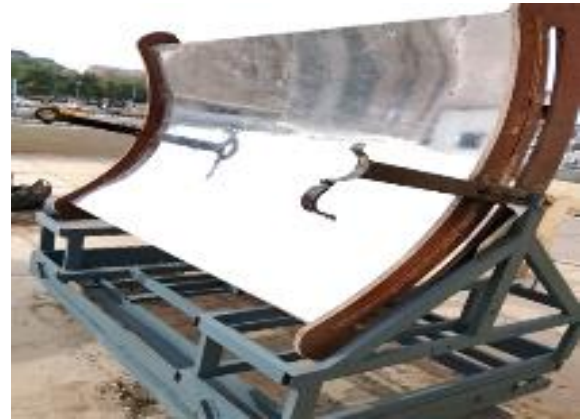
Figure 3: Solar film layer fixed on the top aluminum plate of the reflector surface
