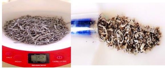
Figure 8. Evacuated tube filling Aluminum metallic medium
