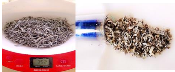
Figure 8. Evacuated tube filling Aluminum metallic medium
