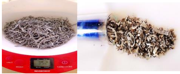
Figure 8. Evacuated tube filling Aluminum metallic medium
