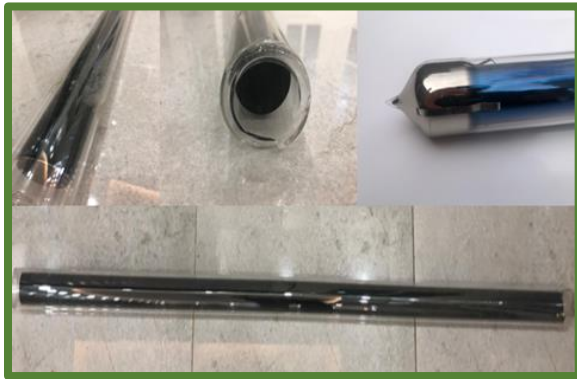
Figure 4: Evacuated glass absorber tube.
