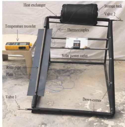
Fig.10. Thermosiphon device [40].
