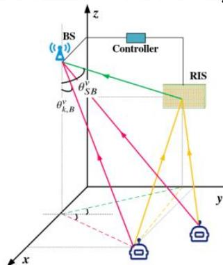
Figure 20 Multi-user localization with the aid of RISs [80]
