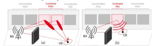
Figure 6 NLoS for both, (a) far-field, (b) near-field wireless positioning with multiple RIS [47]
