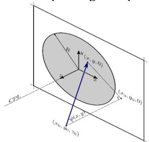
Figure 9 Positioning and transmitting model of the LIS [20].
