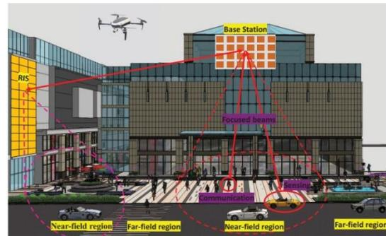
Figure 3 Illustration of near-field communication system.
