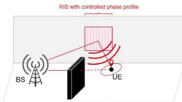
**Figure 7** Single RIS in near field over SISO NLoS downlink positioning scenario.
