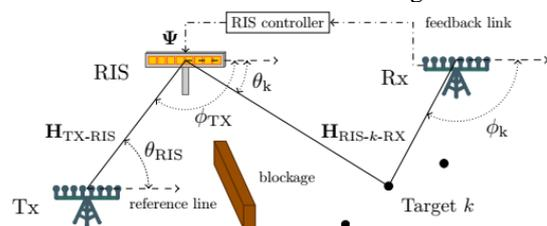
**Figure 18** Multi-target radar system with RIS-aided [78].
