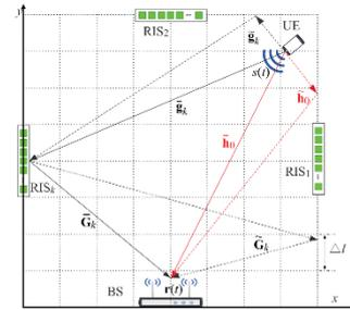
Figure 12 A scenario of distributed RISs assisted indoor positioning [65]
