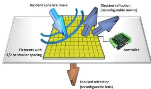
**Figure 1** An example of a RIS in which individual elements are adjusted via a controller [10].
