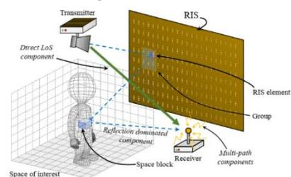
Figure 14 Posture recognition system using RIS [73].
