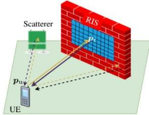
Figure 8 Single antenna UE and RIS system with multipath reflection from passive objects [57].
