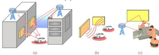
Figure 2 RIS-based positioning applications [43]
