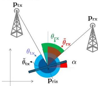
**Figure 16** Single-antenna TX and RX, together with a RIS whose direction and location are unknown [76].
