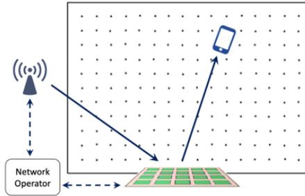
Figure 19 System model for RIS-aided localization [79].
