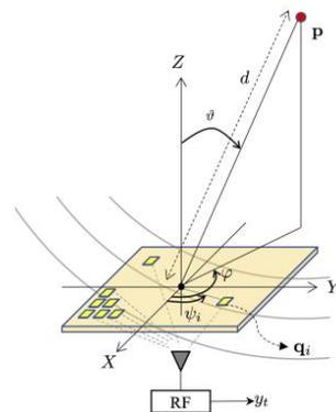
Figure 10 Single UE and RIS lens with a receiving antenna attached to RF chain [60].
