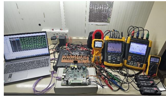
Figure 7. Experimental Setup of the seven-level multilevel inverter
