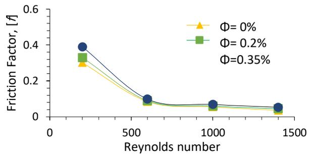
Figure 7. Friction factor for different Reynolds number.
