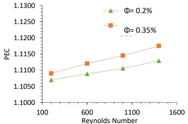
Figure 10. Performance factor of the nanofluid at different Reynolds number.
