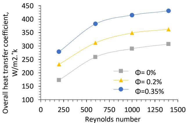
Figure 6. Total heat transfer coefficient at various Reynolds Number.
