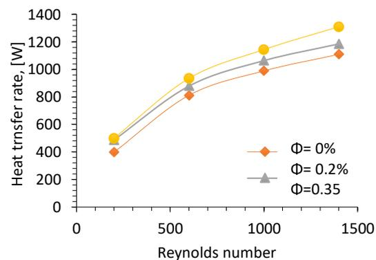
Figure 5. Heat transfer rate for different Reynolds number.
