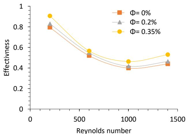
Figure 8. Variation in heat exchanger effectiveness with different Reynolds number.
