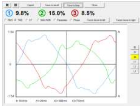
Figure 6: The current waveform measured by a power quality analyzer in the glass tempering factory
