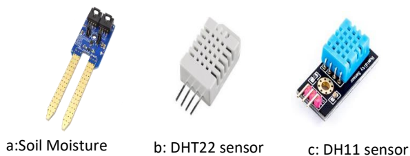
Fig 1. Some of the sensors of smart agriculture
