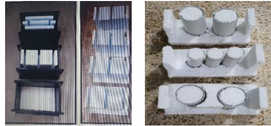
Fig. 4. Details of the dimensions and shape of the cavities inside the concrete blocks
