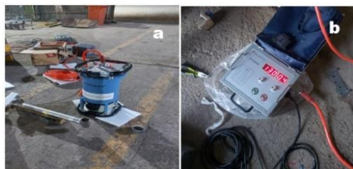
Fig. 4. a) X-Ray Flaw Detector b) Control Panel
