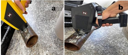
Fig. 3. PMI equipment used: a) SCI Aps x200 b) Sci Aps Z902 C+ Premium
