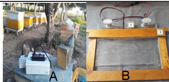
Figure 1. Components of the bee venom milking device A - the electrical transformer b - the wooden frame.
