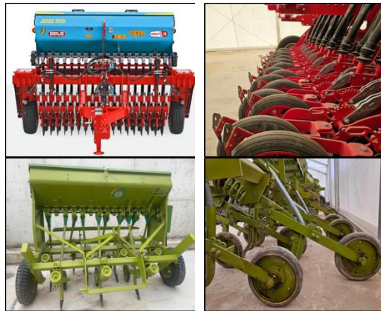
Figure 1. The seeders used in the experiment; (top left) front view of the disc seeder (top right) side view of the press wheels in the disc seeder; (bottom left) front view of the tine seeder, (bottom right) side view of the press wheels in the tine seeder.
