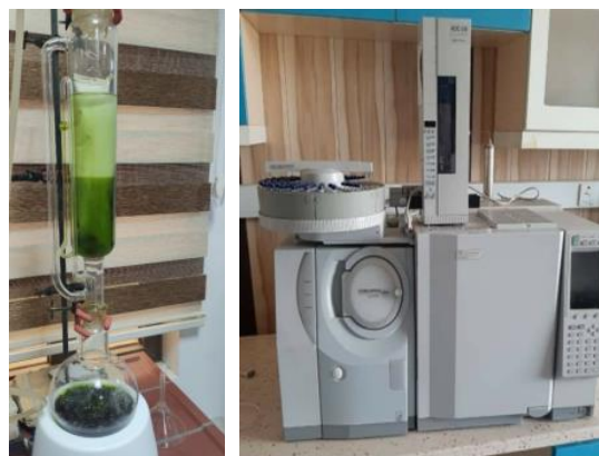
Figure (1A) Soxhlet device, (1B) GCMS-QP2010
